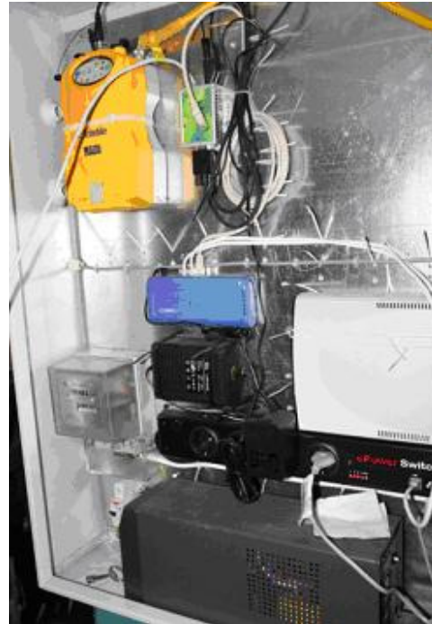
Fig. 2. LitPOS station with Trimble 5700 receiver
