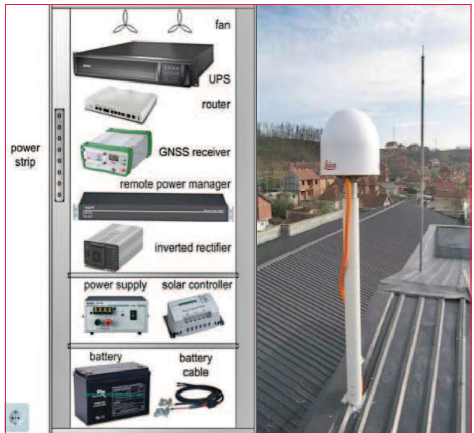
Figure 5: Equipments placed in the cabinet and the GNSS antenna in one of the stations
