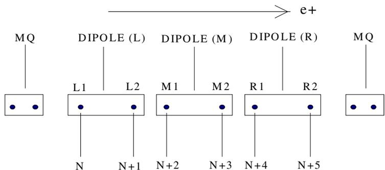
Fig.3 Positions of Dipoles and Quadrupoles
