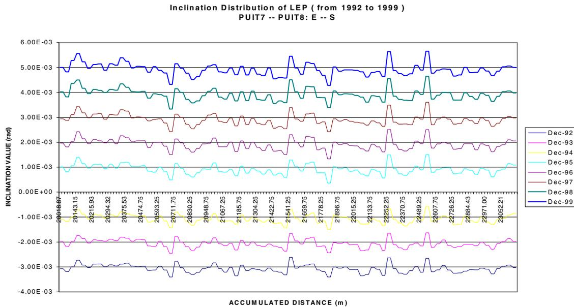
2. The sections 7 and 8 have an evident inclination variation of quadrupoles. The sections 2, 3 and 7 have evident deformation variation following studying on the inclinations of E-S.
