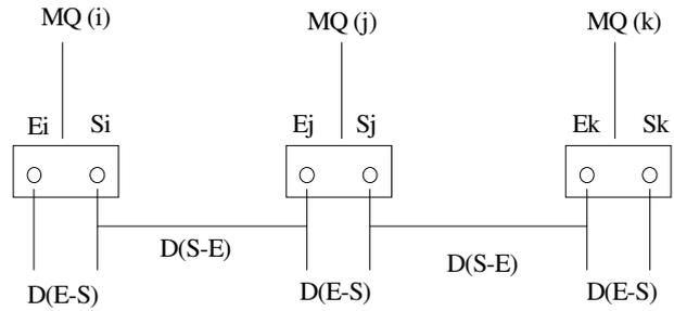
Fig.5 Positions of Quadrupoles
