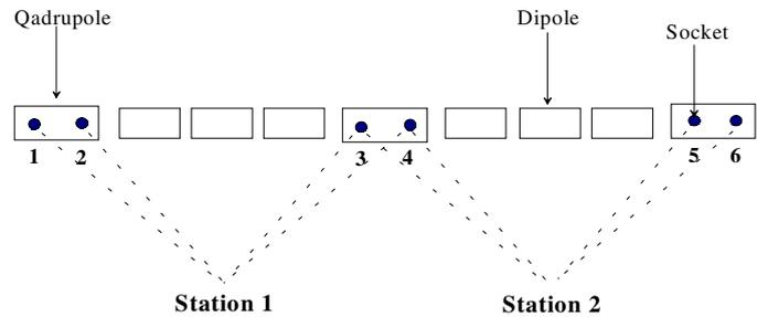
Fig. 2 Method for Leveling of LEP
