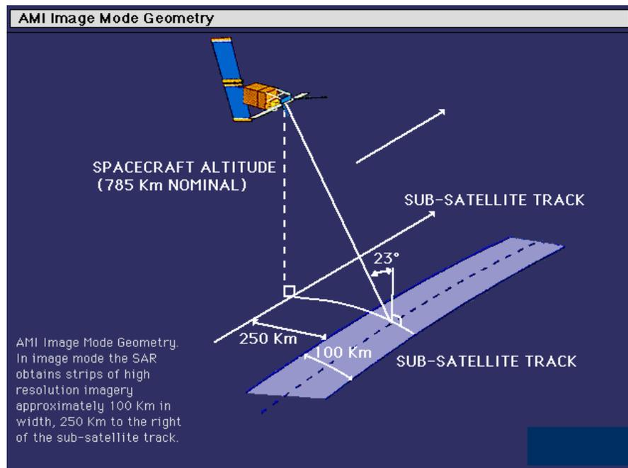
Figure 4. Imaging geometry of ERS satellites (after ESA, 2000).
