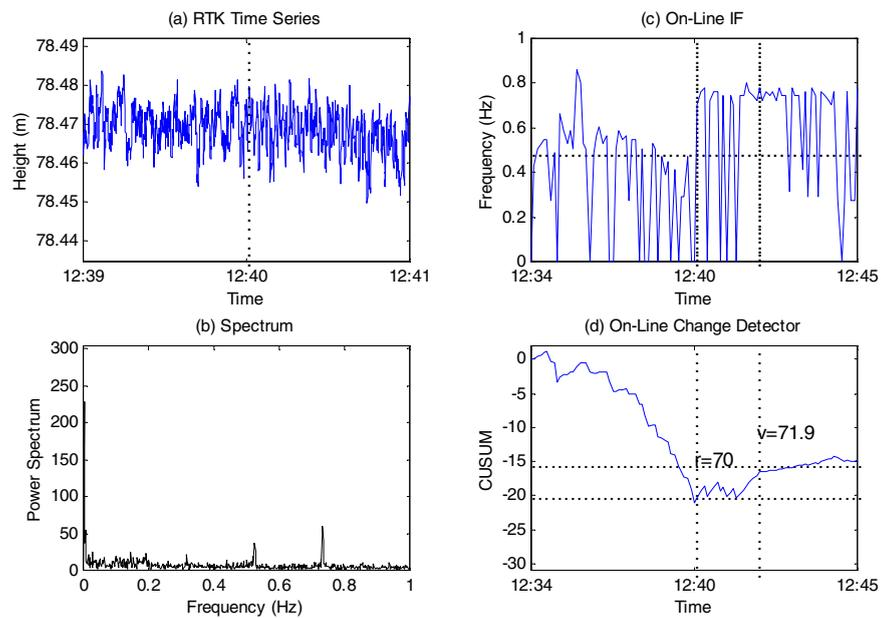
**Figure 6. Low-to-low frequency change (0.5Hz to 0.7Hz at 12:40).** Test parameters: initial mean  $\mu_0 = 0.5\text{Hz}$ ; anticipated shift  $\Delta = 0.1\text{Hz}$ ; threshold  $h = 4$ . Change detected at **12:41**.
