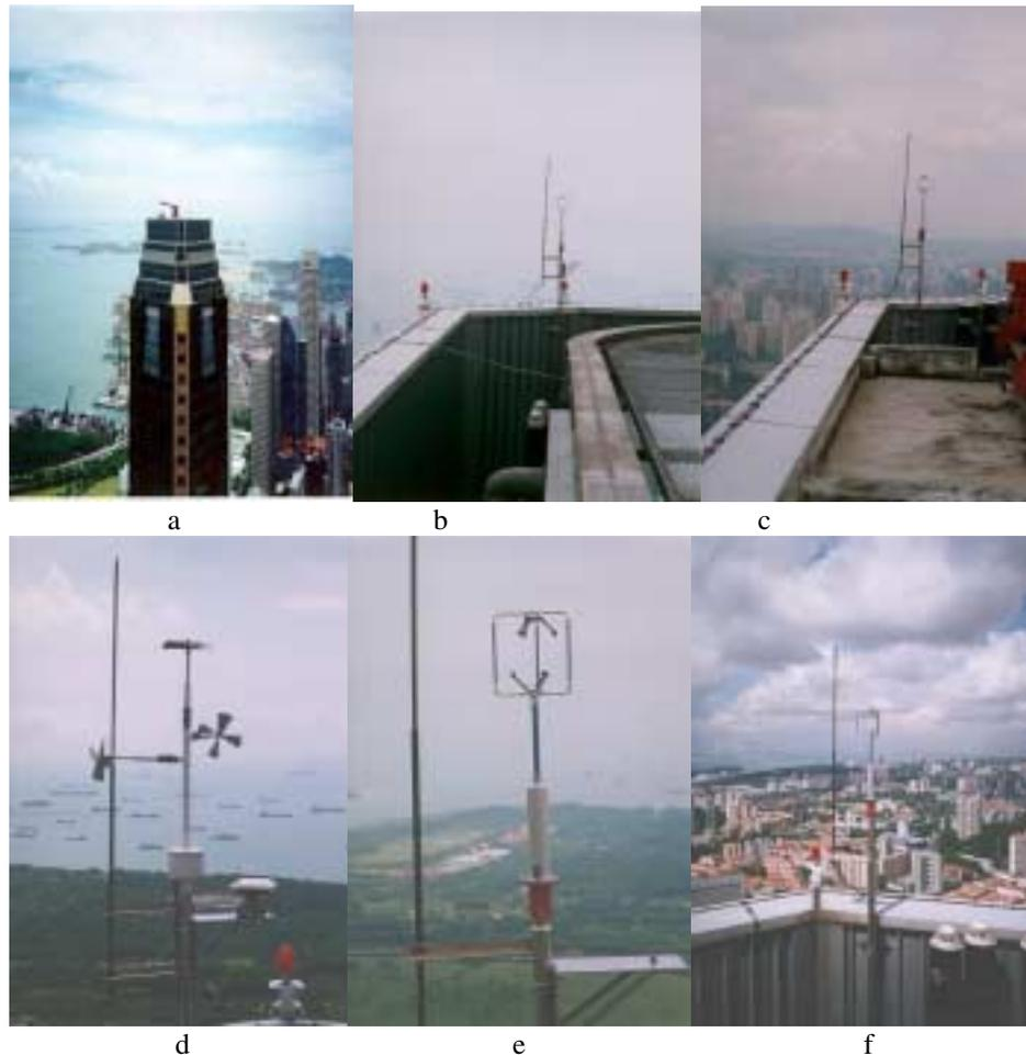
**Figure 3. Existing instrumentation on the Republic Plaza Building:** a) View of level 66 roof/parapet; b) Sonic anemometer at East corner; c) Sonic anemometer at West corner; d) Typical antenna bracket at East corner; e) Close up of West corner; and f) Example of a GPS antenna (with earlier version of anemometer).
