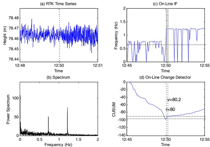
**Figure 7. Low-to-high frequency change (0.7Hz to 1.2Hz at 12:50).** Test parameters: initial mean  $\mu_0 = 0.7\text{Hz}$ ; anticipated shift  $\Delta = 0.45\text{Hz}$ ; threshold  $h = 4$ . Change detected at **12:50**.
