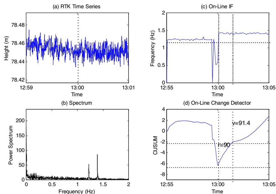
**Figure 8. High-to-high frequency change (1.2Hz to 1.4Hz at 13:00).** Test parameters: initial mean  $\mu_0 = 1.2\text{Hz}$ ; anticipated shift  $\Delta = 0.1\text{Hz}$ ; threshold  $h = 4$ . Change detected at **13:01**.
