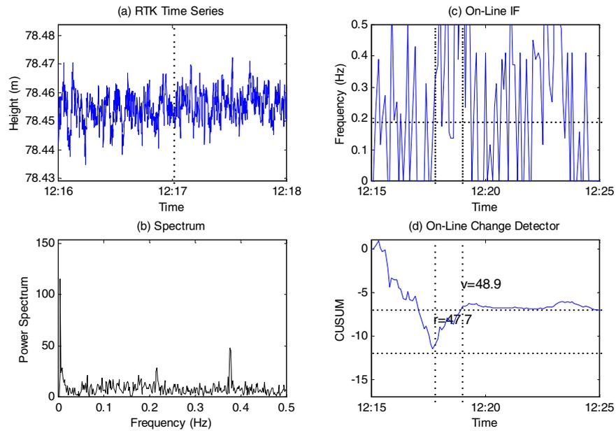
**Figure 5. Low-to-low frequency change (0.2Hz to 0.3Hz at 12:20).** Test parameters: initial mean  $\mu_0 = 0.2\text{Hz}$ ; anticipated shift  $\Delta = 0.1\text{Hz}$ ; threshold  $h = 4$ . Change detected at **12:17**.
