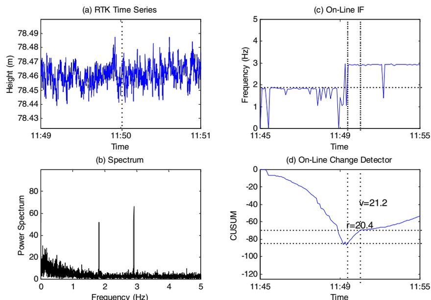
**Figure 4. High-to-high frequency change (2.0Hz to 3.0Hz at 11:50).** CUSUM test parameters: initial mean  $\mu_0 = 2.0\text{Hz}$ ; anticipated shift  $\Delta = 0.5\text{Hz}$ ; threshold  $h = 16$ . Change detected at **11:51**.
