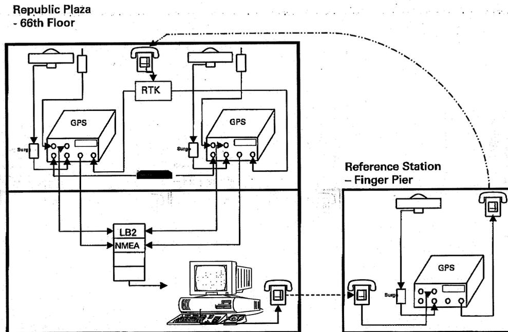
Figure 2. Layout of the GPS monitoring system: one base station at the Finger Pier (PSA Building), two 'rover' stations on the Republic Plaza Building.
