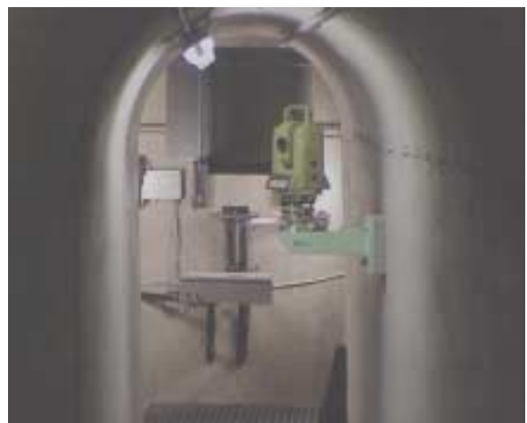
Figure 9 Inverse pendulum chamber with traverse bracket and TC2002
