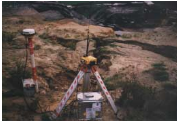
Figure 2: GOCA operating with a Trimble 4600LS receiver and a Trimtalk radio modem in a landslide area
