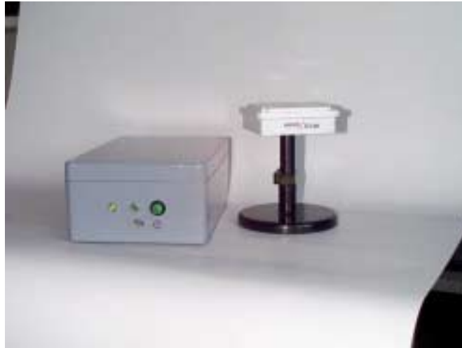
Figure 3: GOCA DGPS-receiver constructed by EuroNav
