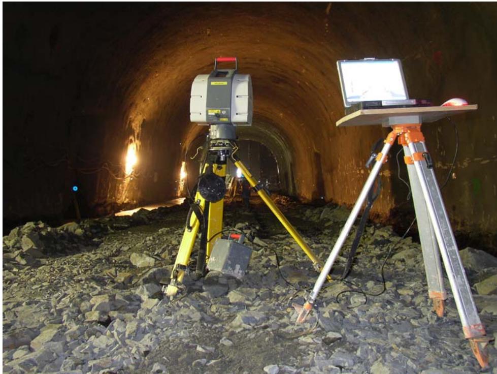
Fig. 1: HDS 3000 laser scanning system
