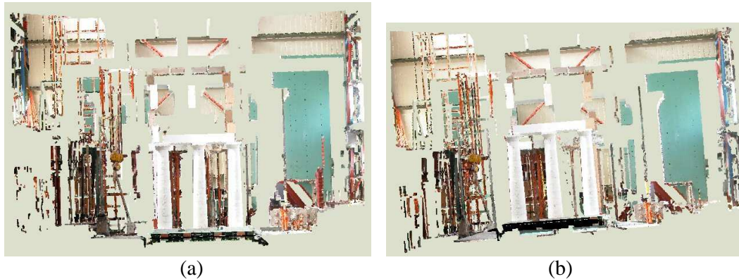
Figure 1 - Scanner acquisitions (a) before and (b) after the earthquake stress
