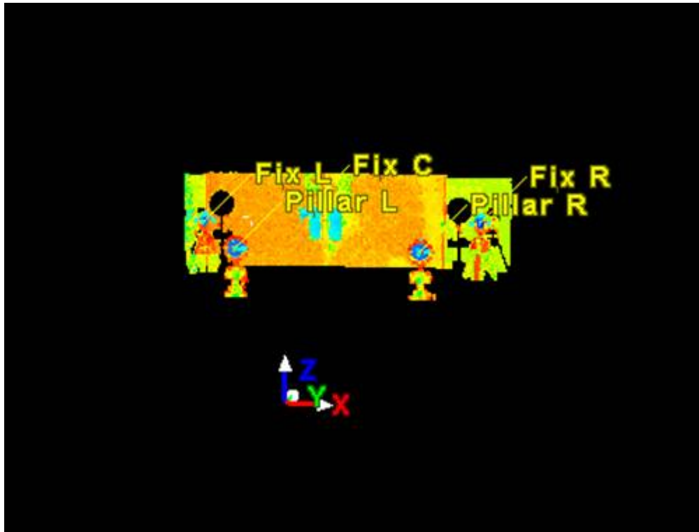
FIGURE 6 , The origin of the scanner axes and target positions in the point cloud.
