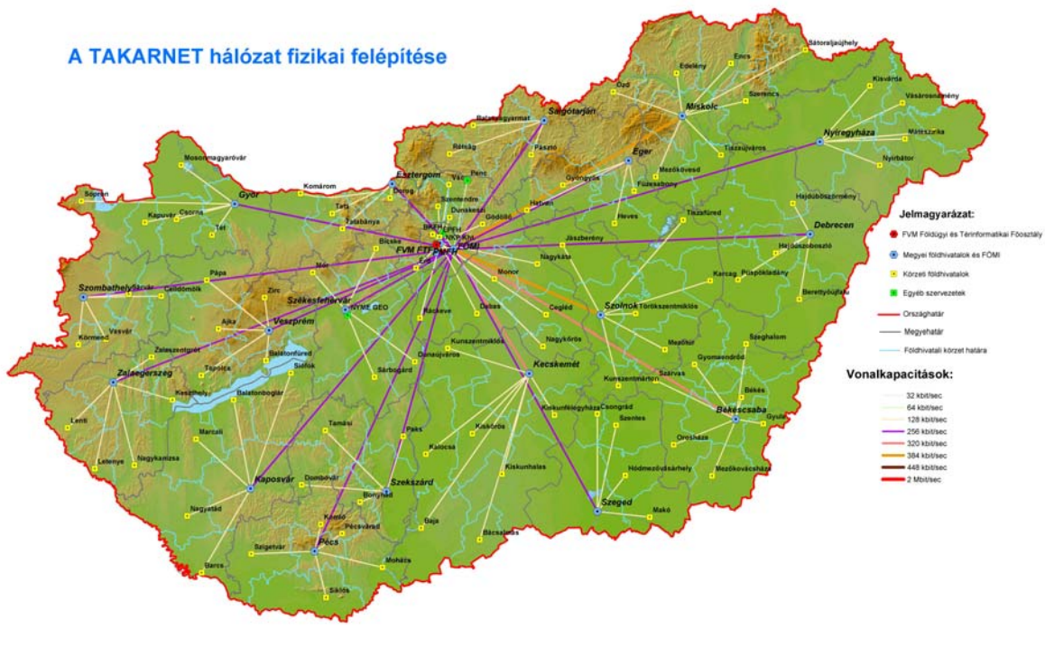
Figure 1.: Physical structure of TAKARNET network
