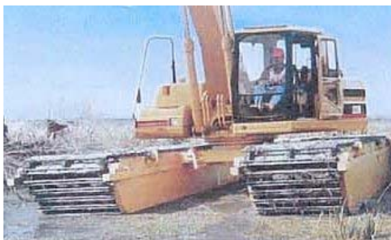
Figure 3B Swamp buggy creating a path into the site for the dredger
