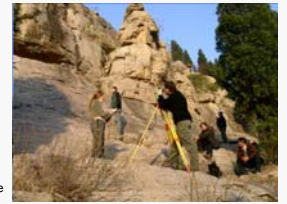
Total Station at northern slope of Hondingshan
