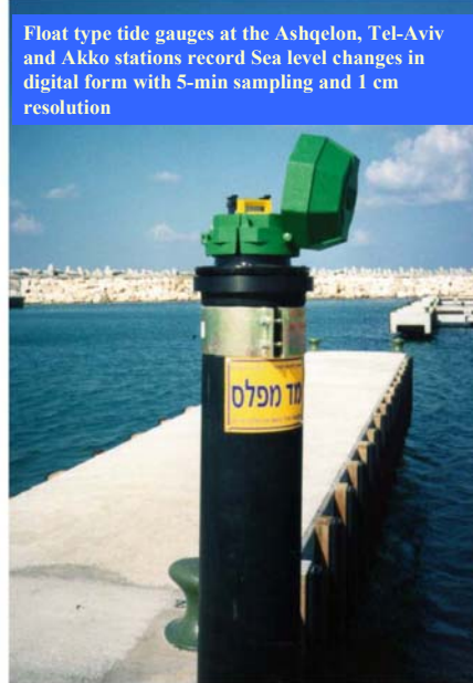
TGBM at the Akko (Acre) station It's height is derived from a local geodetic leveling, it is connected to the national leveling network.
