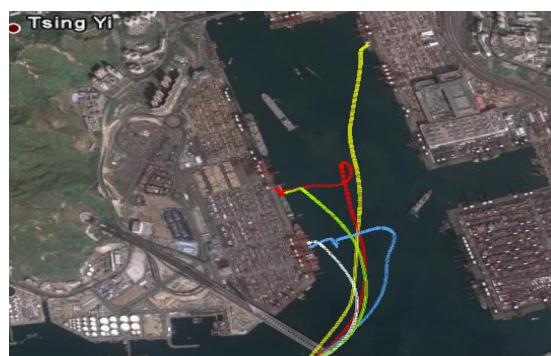
Figure 3 Precise trajectory of the five ships within the docking area. Absolute positions are resolved within 0.1 decimeter error.
