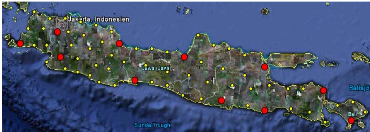
Figure 4. Planned location and distribution of BPN GPS CORS station in Java [Adiyanto and Wibisono, 2009]. Class-A and Class-B stations are denoted with red and yellow circles respectively.
