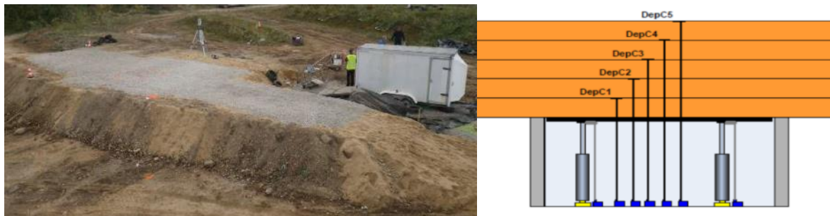
Figure 15: dam mockup and jacks system
