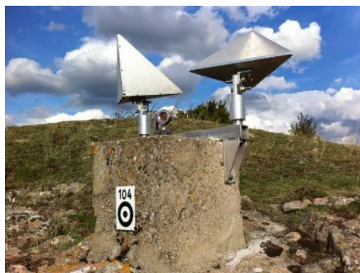
Figure 7: survey point equipped with corner reflector for two modes
