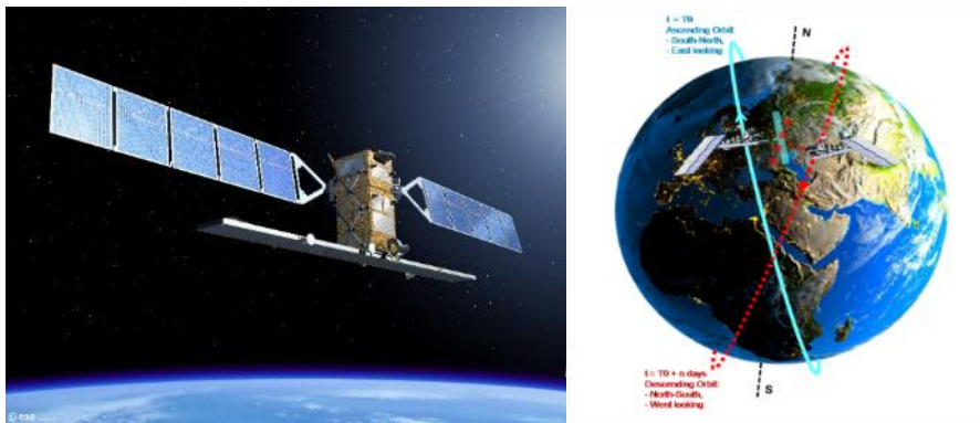
Figure 1: SENTINEL satellites – ascending and descending orbits
