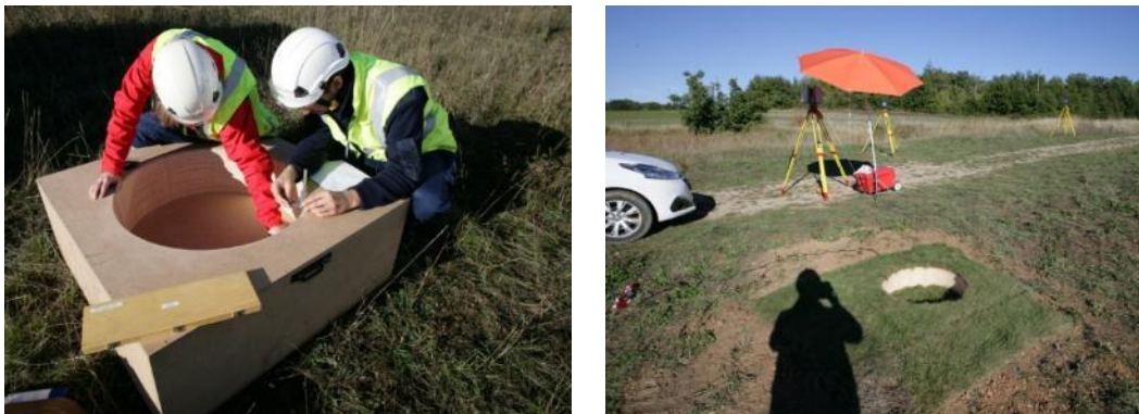
Figure 21: the sinkhole simulator
