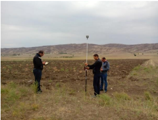
Fig. 1: Survey of boundary with GNSS
