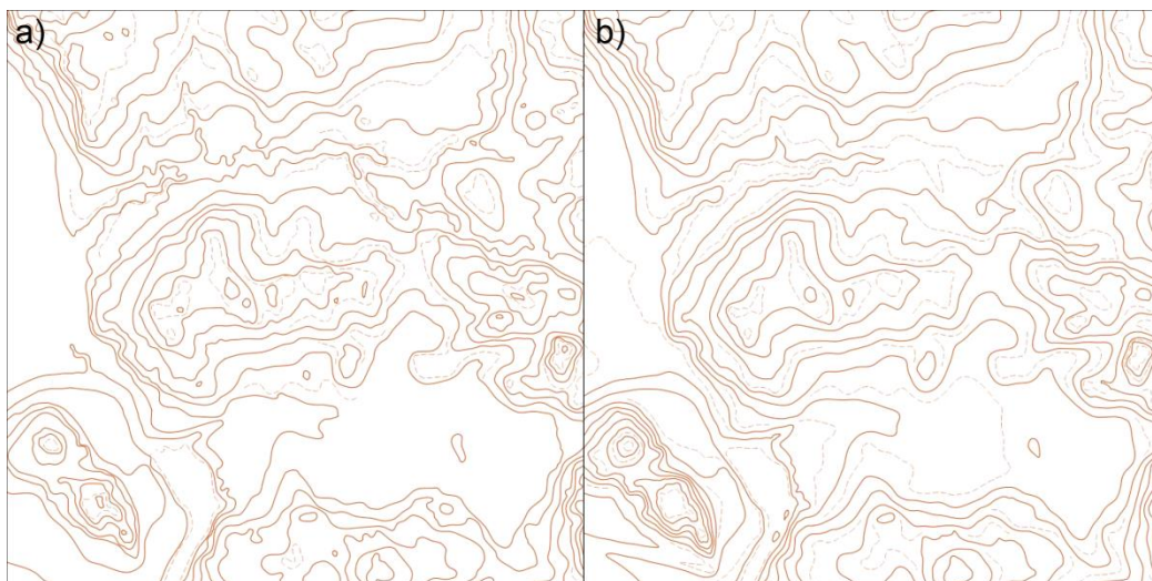
Figure 2. Index/intermediate contours (solid lines) and supplementary contours (dashed lines) from the current manually mapped TDB (a) and from our automatic contouring process (b).
