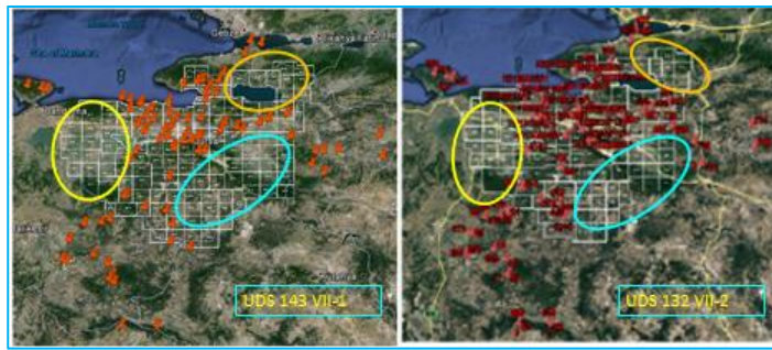
Figure 2 : Unified GCPs sets of 143 and 132 points and distribution to project area M5 and gaps
