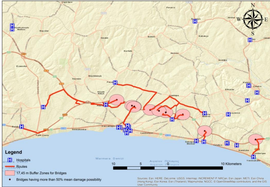
Figure 6. Buffer zones having the value of 17.45 m for bridges
