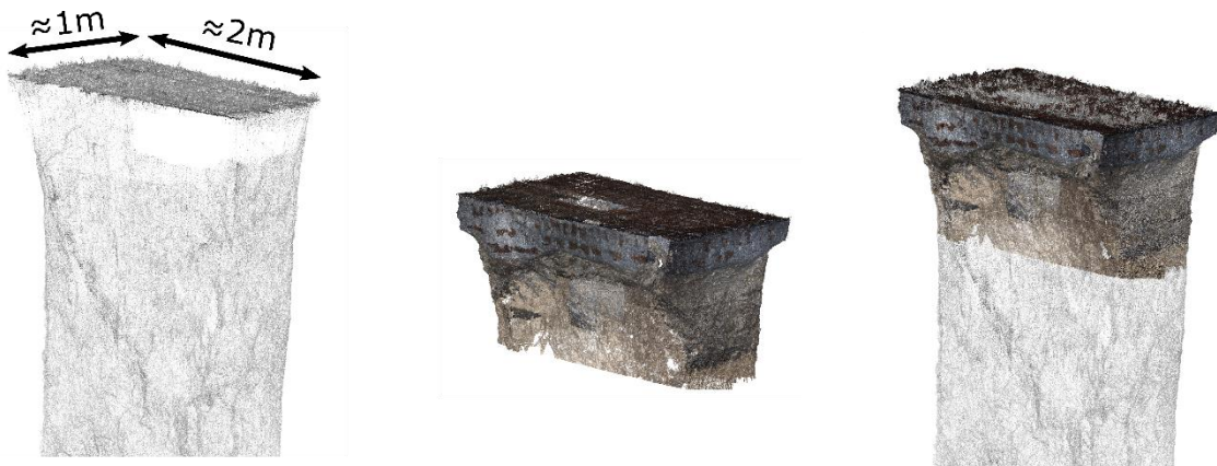
Figure 3: Point clouds of the narrow vertical shaft. Left: TLS point cloud, Middle: photogrammetric point cloud, Right: point clouds combined using the proposed algorithm. For clarity we only show the top part of the shaft and as a negative, i.e. looking at the empty space represented by the point cloud (the shaft seems to be a column).
