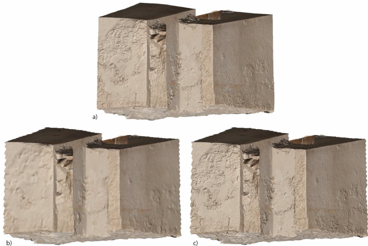
Figure 7: Examples of the rendered 3D-models with different geometric resolution and with the application of the bump map. Figure c) shows a low-density mesh with approx. 22'000 faces where the bump map from the mesh with 25 Mio faces depicted in a) was applied. Figure b) shows the rendering of the low-density mesh without the bump map. The difference is clearly visible when compared to the model with the bump map in figure a).
