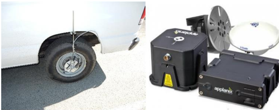
Figure 2: Photo of the 3D laser profilers (LCMS) and INS system on the survey vehicle.
