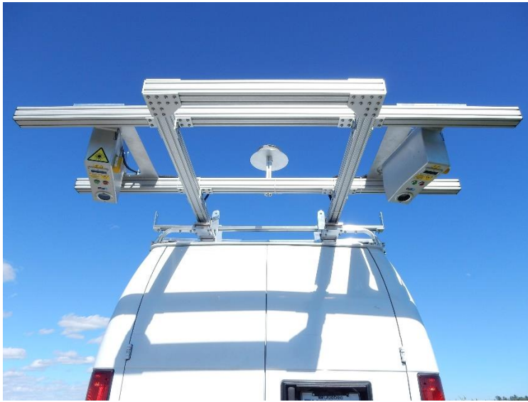
Figure 1: Photo of the 3D laser profilers (LCMS) and INS system on the survey vehicle.
