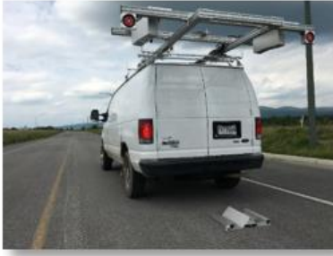
Figure 5: Scan of the calibration object.
