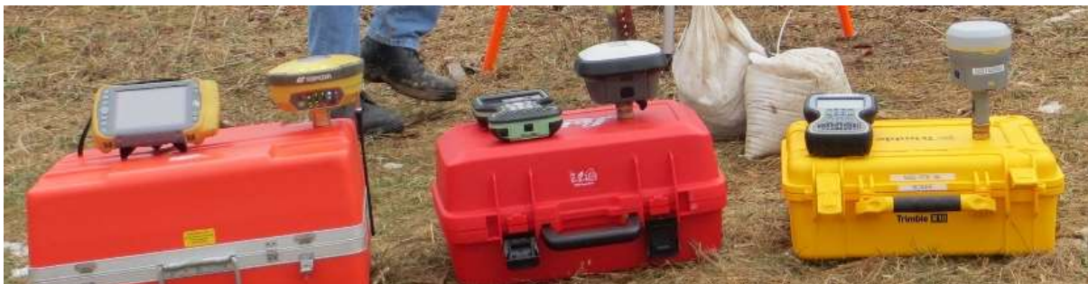
Figure 2. GNSS rovers and data collectors used in the NRTK survey; from left to right: the Topcon Hyper V, Leica GS18, and Trimble R10 integrated GNSS antenna/receiver
