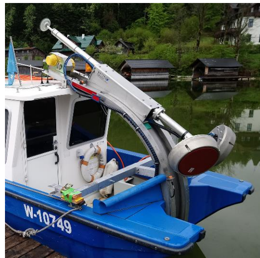
Fig. 2: Survey vessel with Kongsberg EM2040 multibeam echosounder dual head
