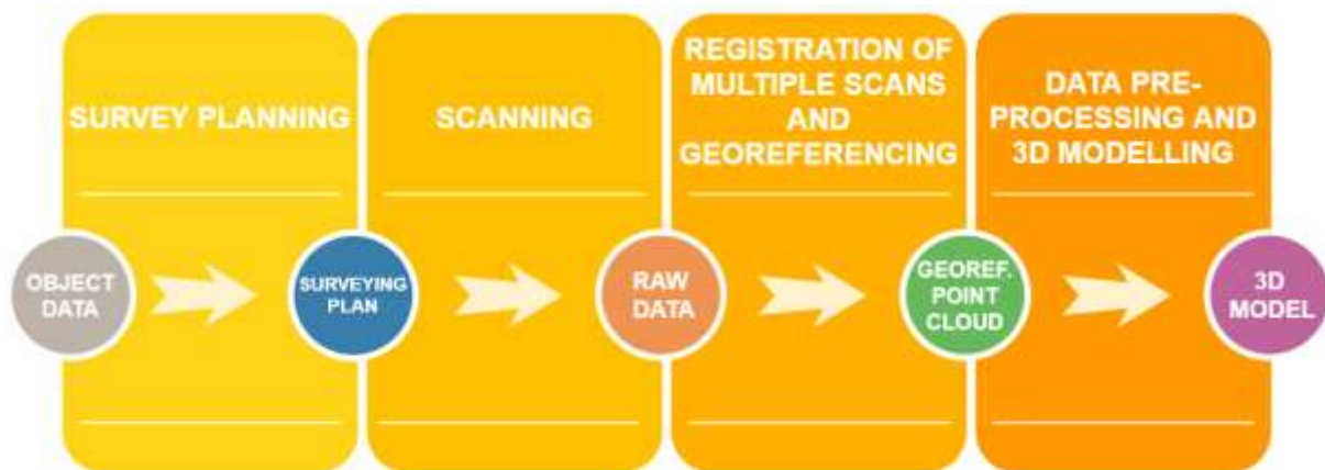
Figure 2. TLS surveying procedure
