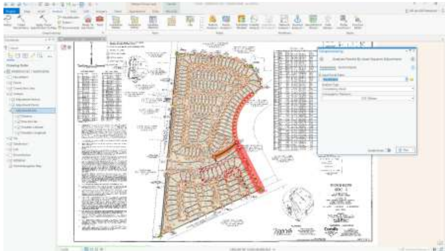
Figure 4: Use of the DynAdjust Least Squares Engine to detect and visualize outliers in a submitted subdivision plan (data courtesy of Harris Appraisal District Texas)
