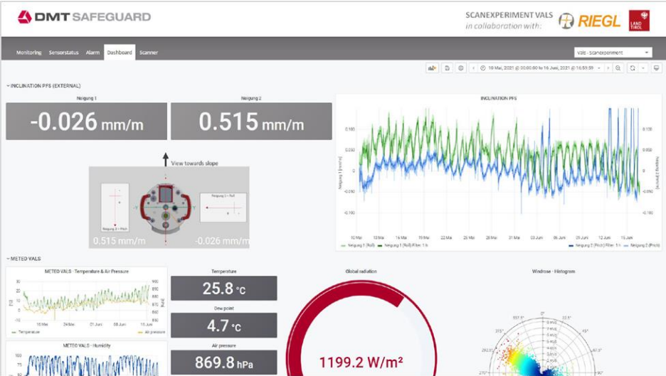
Figure 6: Visualization of the inclination sensor system as well as the weather data in DMT SAFEGUARD.
