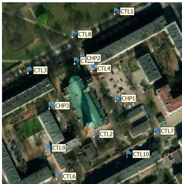
Figure 2: GCP distribution (CTL - control points, CHP - check points)
