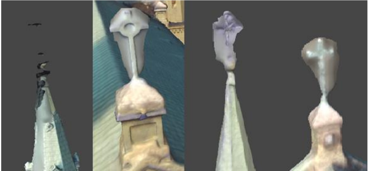
Figure 7: Incorrectly generated mesh model areas
