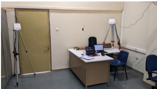
Fig. 10: Deployment of the setup – photo of 2 of the anchors
