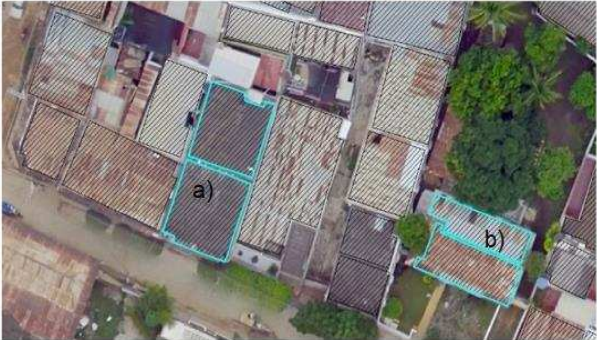
Figure 3. Examples of divided roof into multiple polygons: A). Hipped roofs and, B). Multiple materials.
