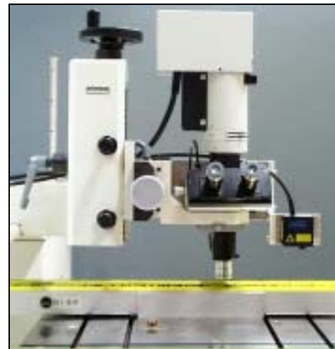
Figure 3: Electro-optical microscope for edge detection
