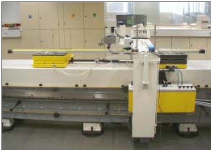
Figure 2: The horizontal comparator for staff calibration at UniBwM
