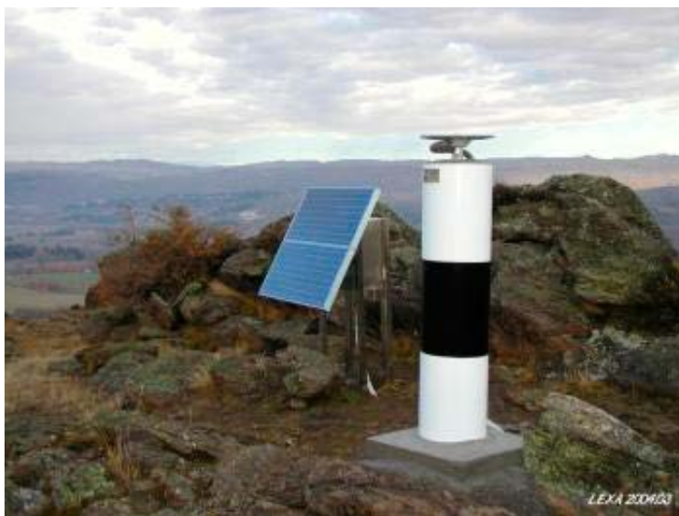
Figure 2: Typical CORS station.
